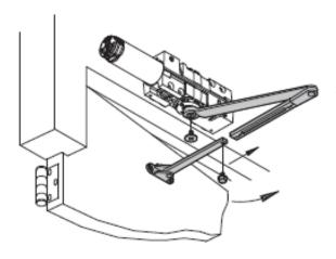
Place the closer arm hex hole onto the bottom of the lower pinion shaft ensuring the two marks (one on the pinion shaft and one on the arm hex hole) align correctly. Once the closer arm is in position use a rubber mallet to gently tap the arm in place fully. Use the 4040XP-159 Arm Screw – Part #4 to secure the installation.
