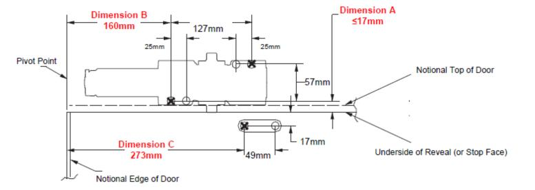
Lateral Mounting Plate Alignment – Dimension B aligns with the left hand most set of drilled and tapped holes, as indicated (see above). This dimension is taken from the centre line of the pivot point of the door.
