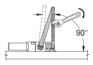
Pre-load the arm to 90° as shown - Rotate the main arm such that the fore arm meets the door at a 90° angle. This will ensure the closer pulls the door fully into the frame once the installation is complete; providing optimum control through the closing arc.
