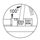
The hex hole at the end of the closer arm engages with the lower closer mechanism pinion shaft at a 100° angle to the closer
