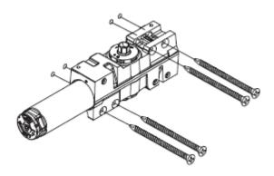
At this stage, do not fix the closer covers in place since you will need access to the hydraulic valves and the spring power dials for final adjustment. Do not adjust the hydraulic valves or the spring power dials at this point.
