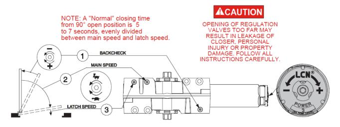
Before attempting to adjust the closer for power or speed open the door back to the maximum angle to check operation. If the door closes fully into the frame in a satisfactory manner, you do not need to make any adjustment.
