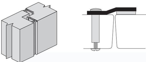
The rebate may be a part of the door construction (commonly found on pairs of timber doors) or it may be a 'plant-on' rebate or 'astragal' introduced as a lock protector or a weather strip. In each instance, in order to effect correct door control, it is necessary always to ensure that the active leaf (or first opening leaf) is the second leaf to close.
