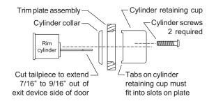
For TP and TP-BE trim on 1-3/4" thick door, cut 1/4" off humbpiece.
