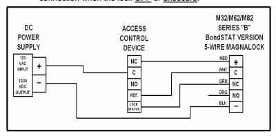
Figure 21. Connections for BondSTAT "B" Version
