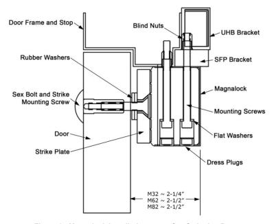
Figure 2. Magnalock Installation on an Out-Swinging Door
