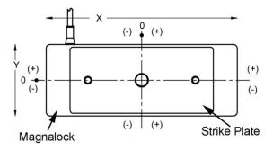
Figure 19. Magnalock and Strike Plate Alignment
