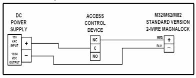
Figure 20. Typical Magnalock Wiring
