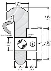
• (5/16" diameter x 1" long throw bolt) and one 1/2" thick sponge neoprene bottom seal with double faced adhesive for attachment (non-handed)
