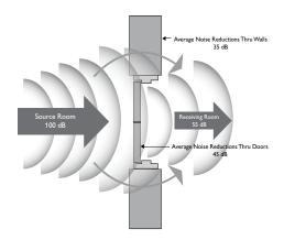
In order to reduce the transmission of sound, materials are added between the source room and the receiving room. The resulting change in decibel level is the sound transmission loss and is given a Sound Transmission Class (STC) rating.
