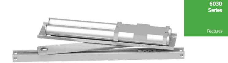
The concealed 6030 Series PACER<sup>®</sup> is a heavy duty, double acting closer designed to fit in a narrow, minimum 1-3/4" header. The single lever arm and roller assembly provides smooth, quiet door control and the choice of finishes and track functions meet virtually all architectural requirements. Installation at left illustrated with center pivot set (not included).
